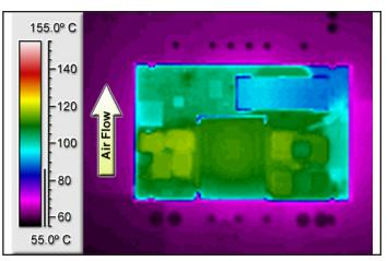
Figure 6: Thermal plot of converter at 23.3 A load current (279.6 W) with 55 °C air flowing at the rate of 200 LFM. Air is flowing across the converter from pin 3 to pin 1 (nominal input voltage).
