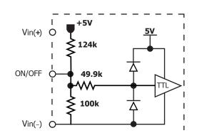
Figure B: Internal ON/OFF pin circuitry
