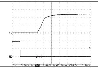
Figure 10: Turn-on transient at zero load (2 ms/div). Load cap: 3 mF output capacitance. Ch 1: Vout (5 V/div), Ch 2: ON/OFF input (2 V/div).
