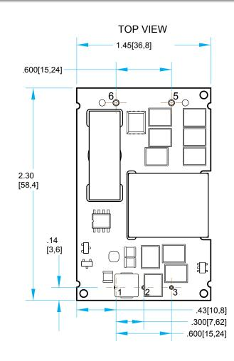
**Open Frame Mechanical Diagram**
