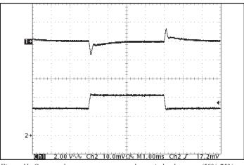
Figure 11: Output voltage response to step-change in load current (50%-75%-50% of lout(max);  $dI/dt = 0.1 A/\mu s$ ). Load cap:  $100 \mu F$ ,  $100 m\Omega$  ESR tantalum cap and 1  $\mu F$  ceramic cap. Ch 1: Vout (2 V/div), Ch 2: lout (10 A/div).
