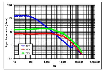
Figure 21: Magnitude of incremental input impedance (Zin = Vin/Iin) for minimum, nominal, and maximum input voltage at full rated power.
