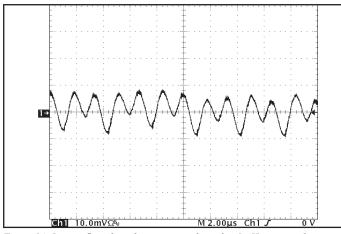
Figure 14: Input reflected ripple current, is, through a 5  $\mu$ H source inductor, using a 47  $\mu$ F electrolytic input capacitor (10 mA/div). See Figure 12.
