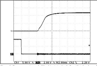
Figure 9: Turn-on transient at half load (resistive load) (2 ms/div). Load cap: 3 mF output capacitance. Input voltage pre-applied. Ch 1: Vout (5 V/div), Ch 2: ON/OFF input (2 V/div).
