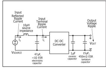
Figure 12: Test set-up diagram showing measurement pints for Input Terminal Ripple Current (Figure 13), Input Reflected Ripple current (Figure 14) and Output Voltage Ripple (Figure 15).
